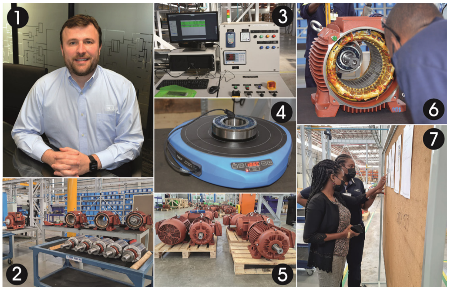
1: Eduardo Werninghaus, CEO at Zest WEG. 2: WEG motors in different phases of the process. 3: Test panel utilised to test all assembly motors. 4: Bearing heater used to prepare bearings for the assembly process. 5: Motors ready for the paint booth. 6: The very first rotor being positioned. 7: Sindi Mbhalati, Operations Executive at Zest WEG (right) and a colleague at the assembly line, during the process of the first motor being produced.
