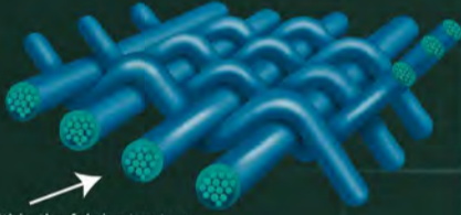
FR pigments within the fabric structure
