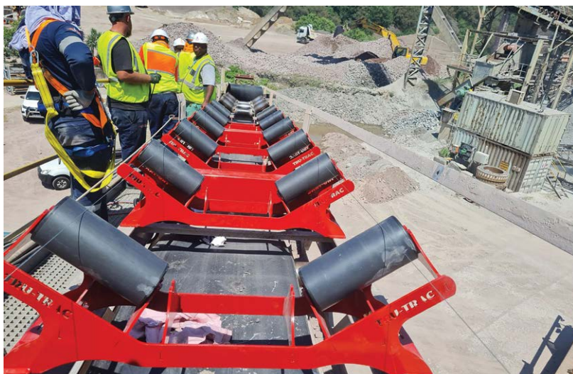
Tru-Trac's flagship TTR FI-4 belt scale system installed at AfriSam Coedmore uses a fully floating pivotless weigh frame supported by four load cells.
