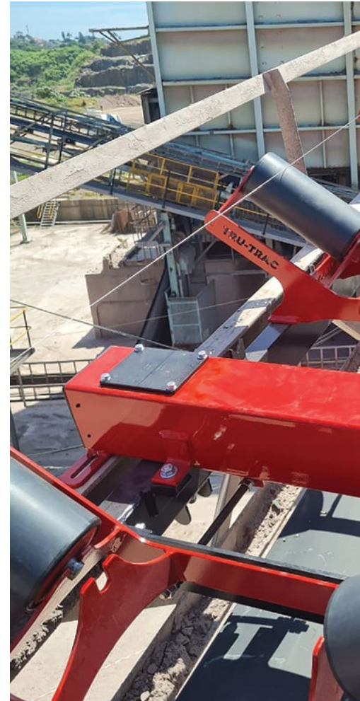
Tru-Trac's shock absorbent and locally produced load cells, designed for durability and quick replacement.
