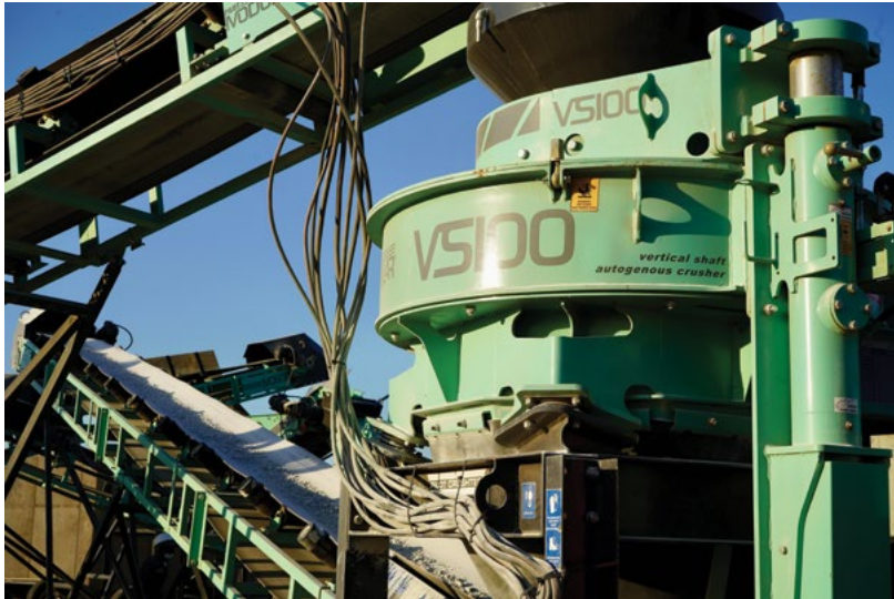
The Twister VS100 is the latest generation of static VSI crusher and is a robust and reliable skid mounted vertical shaft impact crusher, for use in tertiary and quaternary crushing applications.
