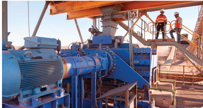
The intelligent platform is used to monitor bearing hydraulics, drive train and tyre wear on Enduron high pressure.
