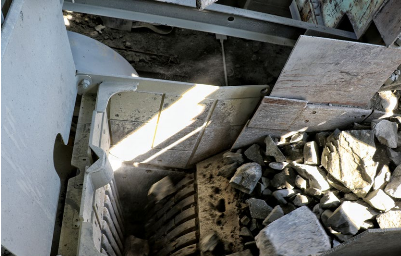
The new addition reduces downtime and is safer to operate and has hydraulic gap adjustment which negates the need to physically adjust gaps. In addition, it is more maintenance friendly.
