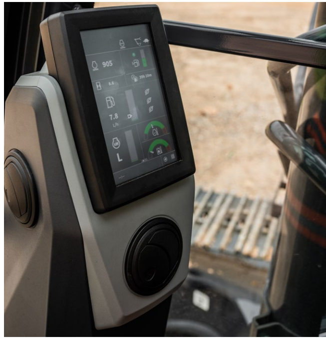
The seven-inch touch-screen monitor provides the operator with quick access to the machine's features, functions and diagnostics.
