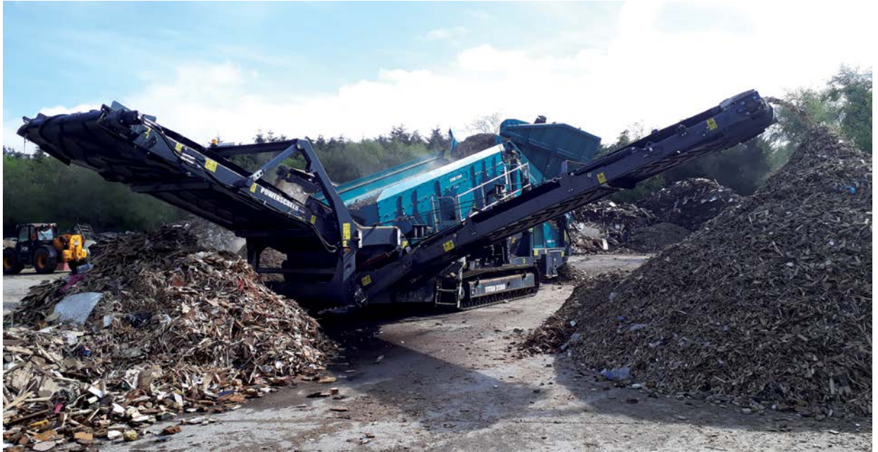
Hybrid Dual Power is available on the Titan 2300, being powered using standard diesel or connected to an external electricity supply once the machine has been set-up.
