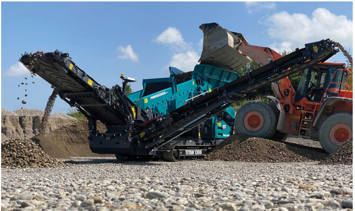
The Titan 1300's highly aggressive screenbox has a total screening area of 10 m 2 .
