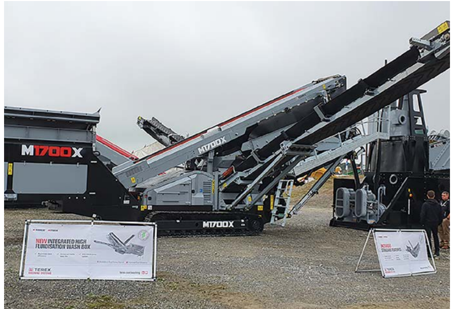
The improved M1700X features a new integrated high fluidisation wash box to maximise deck efficiency, increase media wear life and have an adjustable spray system.
