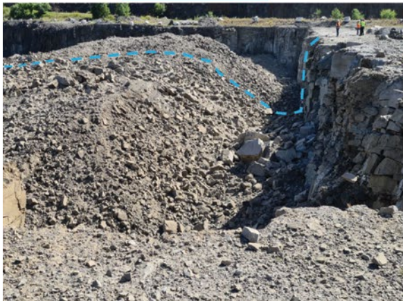
Comparison of muckpile fragmentation between a Varistem and standard blast design.
