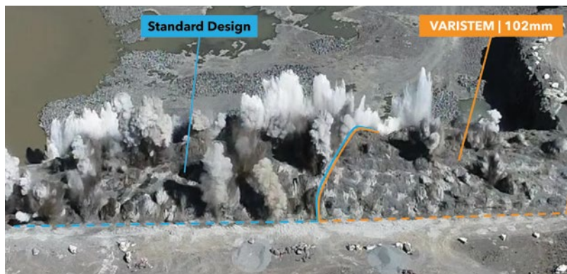
The blast analysis clearly indicated that the time to stemming movement of the Varistem side of the block was multiple times longer than on the non-Varistem side of the block.
