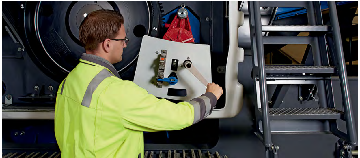
The EUROTEST-certified "Lock & Turn" system provides the highest level of safety during rotor ledge change at the mobile impact crusher and when releasing bridging.
