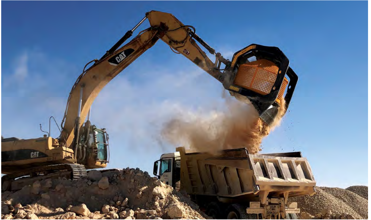
Bucket crushers and bucket screeners from MB process any extracted materials, even the hardest and toughest ones.
