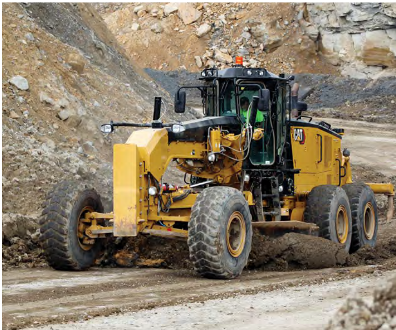
A motor grader driven by a trained operator is crucial for clearing and grading haul roads and most critical to keep the haul road's rolling resistance to a minimum.
