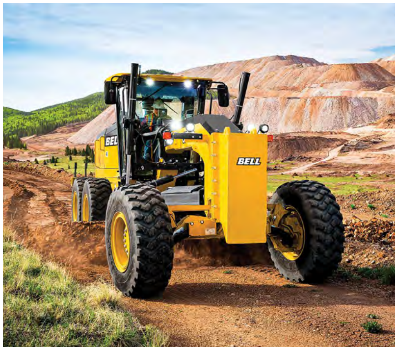
Bell graders have a blade float function that allows the operator to position the blade to just grade the surface.
