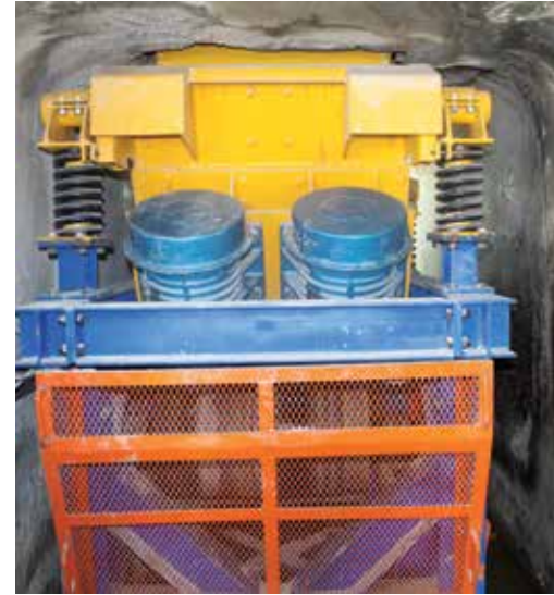
Manual feeding at the tunnel was an impediment to the secondary crushing process, and was addressed by installing a new pan feeder manufactured and supplied by Weir Minerals.
