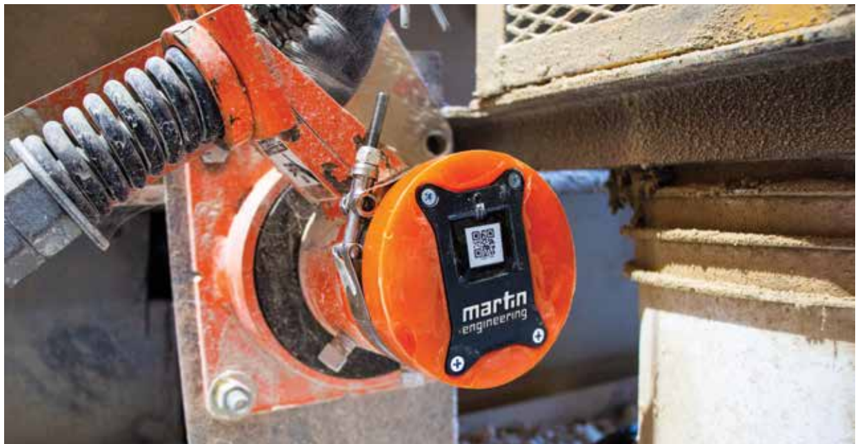
The N2 PI notifies service personnel when a cleaner requires re-tensioning or replacement.
