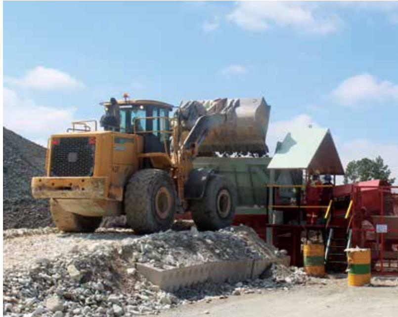
OMV Stilfontein previously experienced loading constraints at the dump, which were addressed by installing a new feeder box and extending the conveyor belt.
