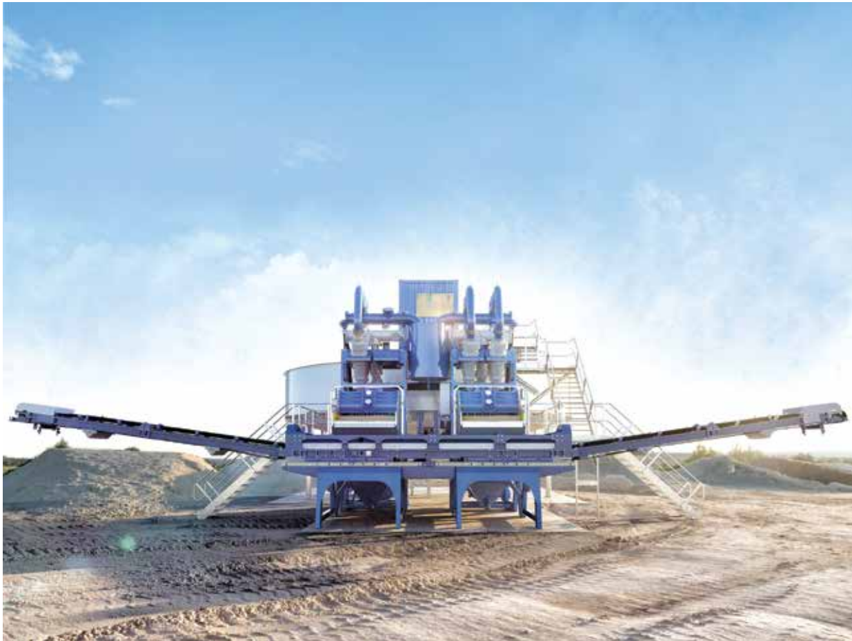
The Combo X900 enables materials processors to wash more than 500 tph.
