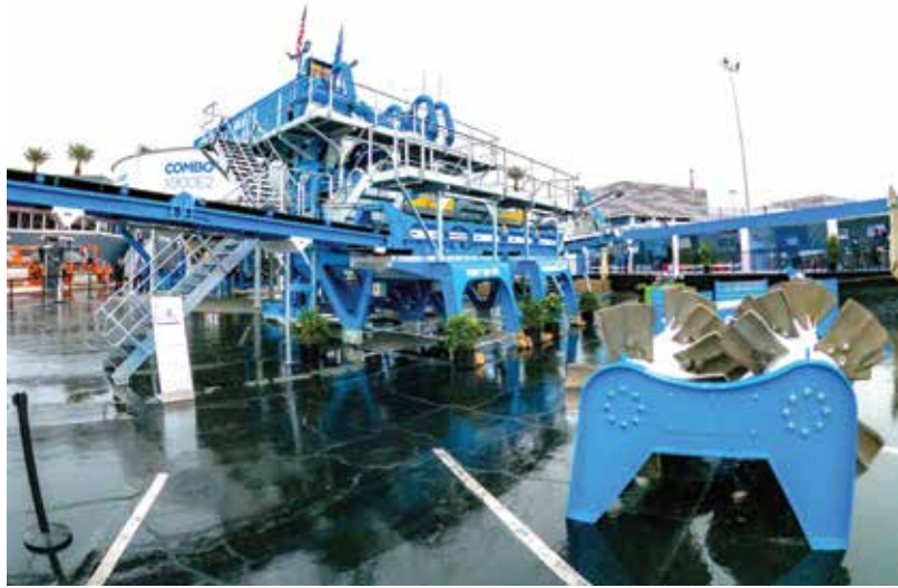
The CDE Combo X900 encompasses five processes – feeding, sizing, sand washing, stockpiling and complete integrated water management.
