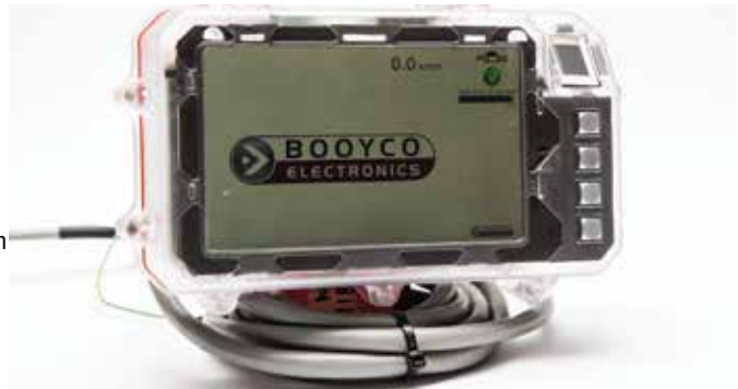
Booyco Electronics’ TMM’s control unit indicates when the vehicle needs to slow down or stop, using audio visual displays.
