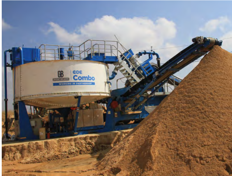
CDE developed and built a Combo modular plant to transform 60 tph of raw feed into washed 0 – 6 mm river sand and 0 – 1,5 mm plaster sand.
