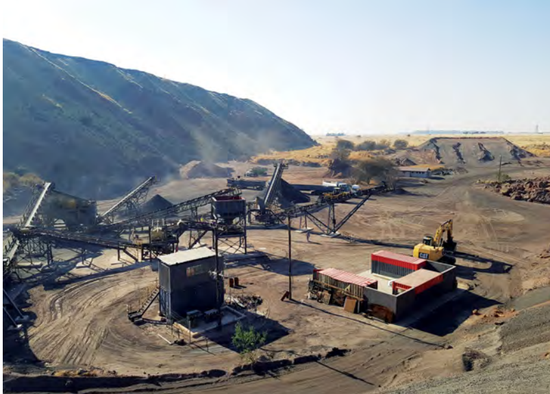
Clinker Supplies produces aggregates through recycling and reclamation of old ash dumps.
