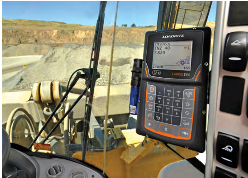
Measurement tools like LOADRITE loader scales give quarry managers real time information about the amount of materials going into or taken out of the stockpile.
