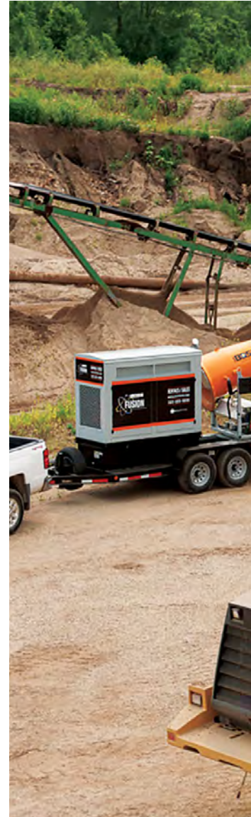
The DustBoss DB-60 Fusion Dust Control and Suppression Cannon from Boss-Tek.
