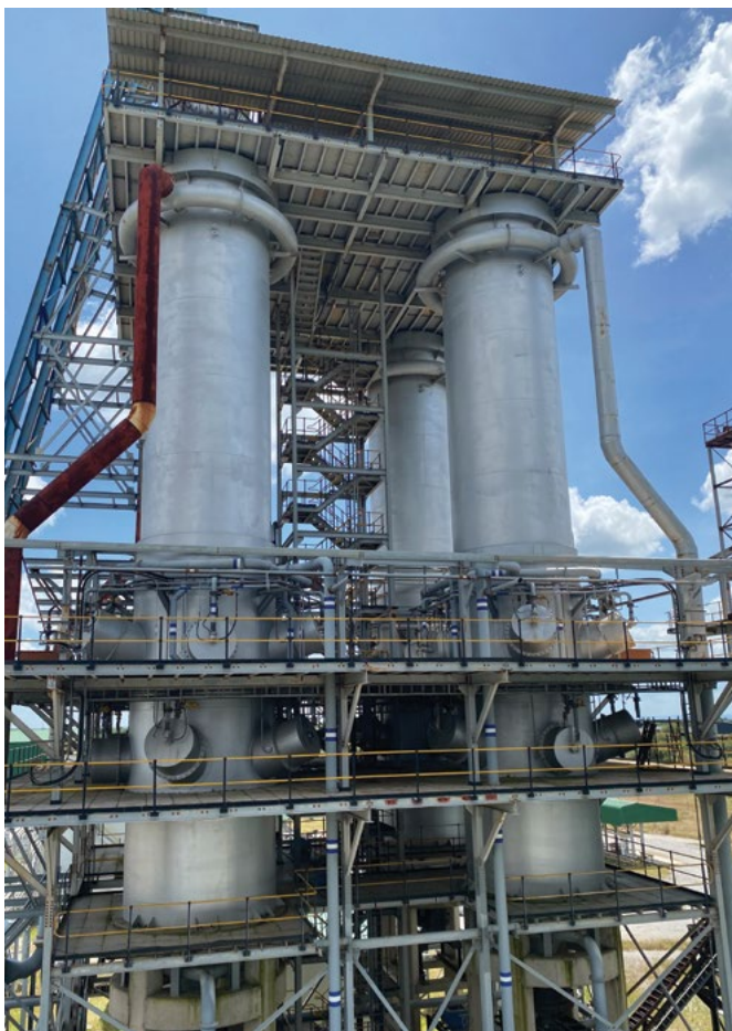
View of the vertical kilns, used for burning the crushed limestone to produce the quicklime product.
