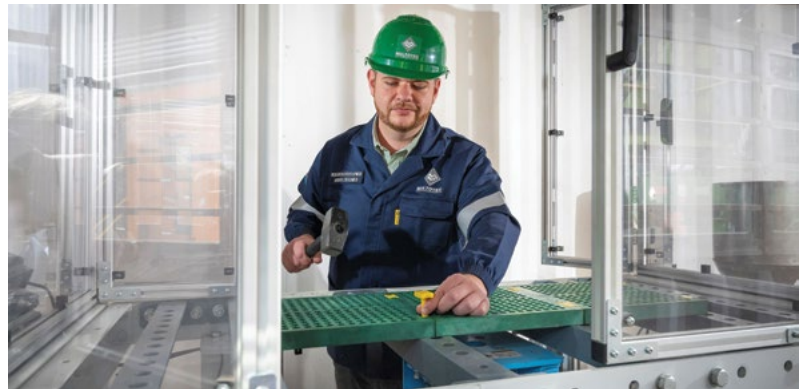
Multotec tests screening media materials such as rubber, polyurethane, wedge wire with various apertures, and thickness.
