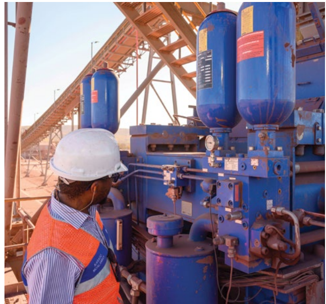
The ENDURON HPGRs are used in crushing applications for fine grinding and use significantly less energy and water than traditional methods.
