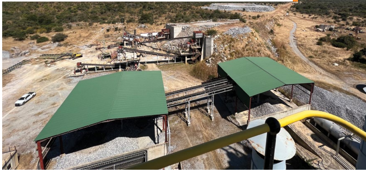
View of the primary crusher, installed at Limeco as part of the 2-stage crushing circuit.
