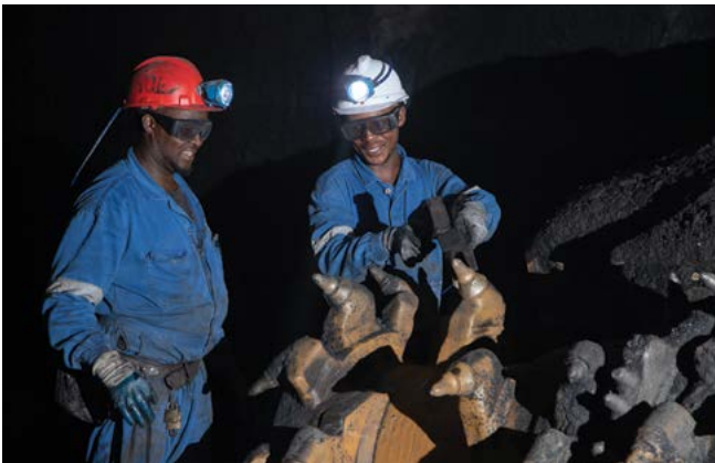
Members of the Kangra team conduct routine maintenance checks on a continuous miner underground.
