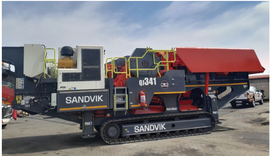
The Sandvik QJ341 mobile jaw crusher has a production capacity of 400 tonnes per hour.
