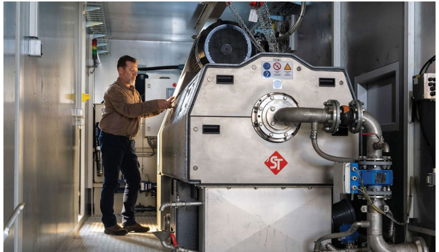
The decanter centrifuge from Multotec comes in a 40-foot container and occupies a small footprint.
