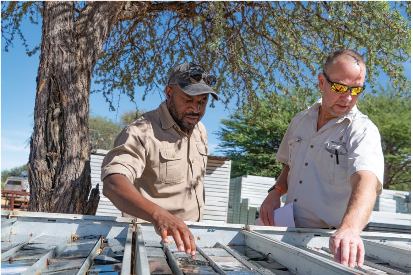
Project manager, Mike Stuart and a team-mate from Omico Mining inspect core samples.
