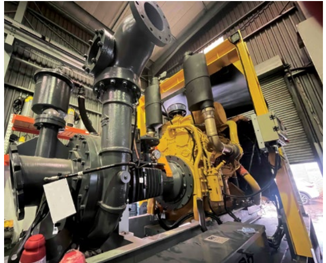
The PAC SH high head pump is built to handle high concentrations of solids and abrasive materials, making it well suited to demanding site conditions.
