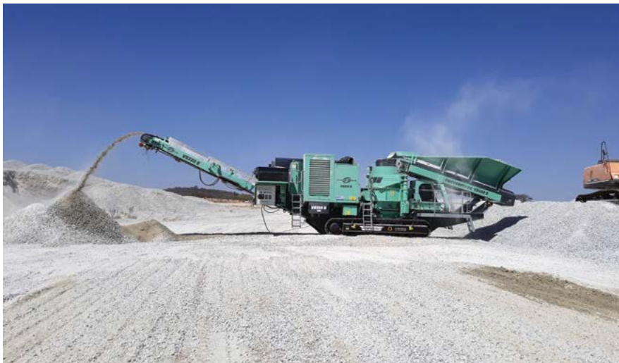
The TwisterTrac VS350E delivers high quality cubical aggregate for mining, quarrying, recycling and construction.
