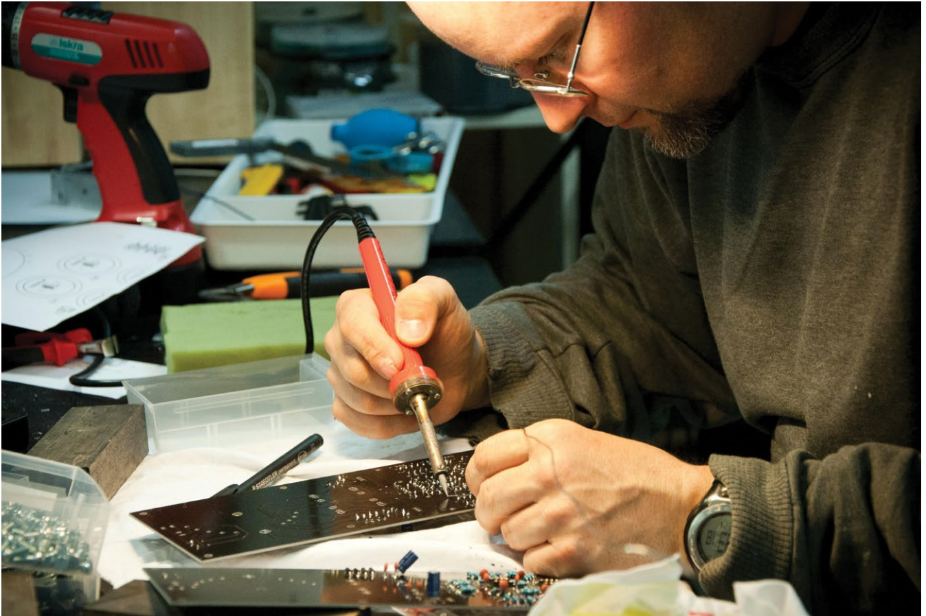
Tin alloys are often used as solder - essential for fusing circuit board components together.
