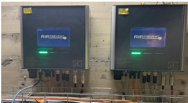
Rip Prevent+ is the first rip detection system for fabric belts, designed without sensor elements inside the belt for universal conveyor application.
