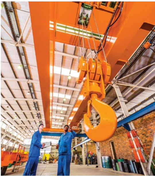
A 20-metre-span Condra crane refurbished for a mine.
