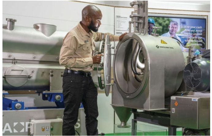
The Tema Process dryer can operate at product temperatures up to 400 °C using various mediums such as air, steam, and inert gas.
