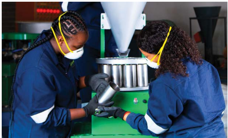
MetSop employees checking the efficiency of the rotary splitter.
