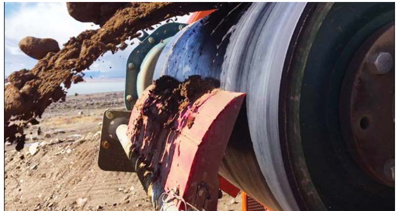
Tru-Trac’s range of trackers employs a unique action that reacts immediately correcting belt misalignment.
