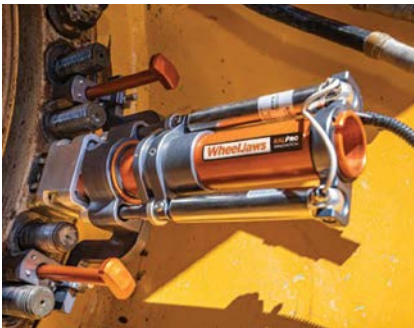
Kal Tire offers WheelJaws - secure, remote-controlled clamps for safe tyre removal.
