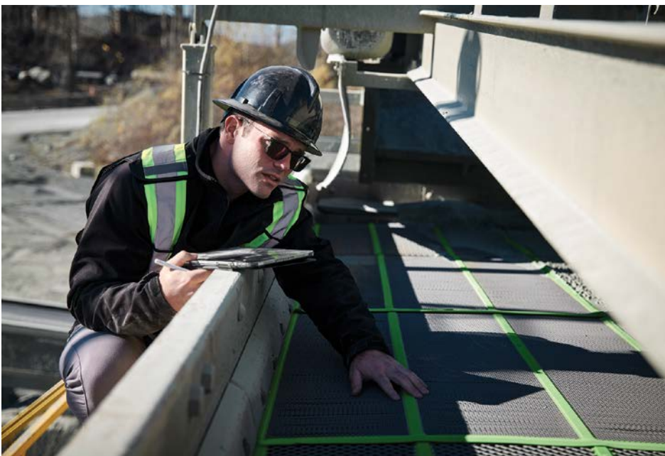
Below: Innovative high vibration media styles allow infinitely minute adjustments of wire spacing to accommodate a plethora of specification requirements.
