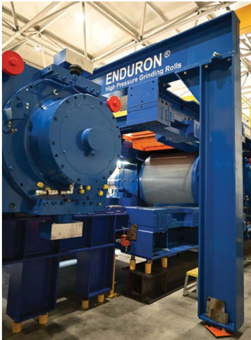
HPGRs require no grinding media or additional water, lowering the environmental impact of the equipment.
