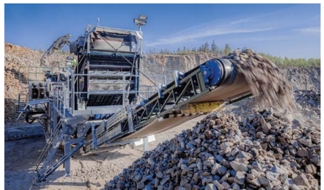
The Jonsson L120-330 includes a primary jaw crusher, cone crusher and screen on the same set of tracks.
