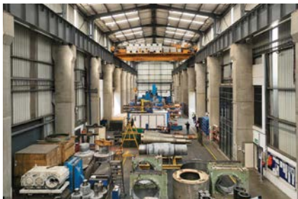
The main workshop at the FLSmidth Chloorkop Service Centre with a HPGR stripped ready for inspection.
