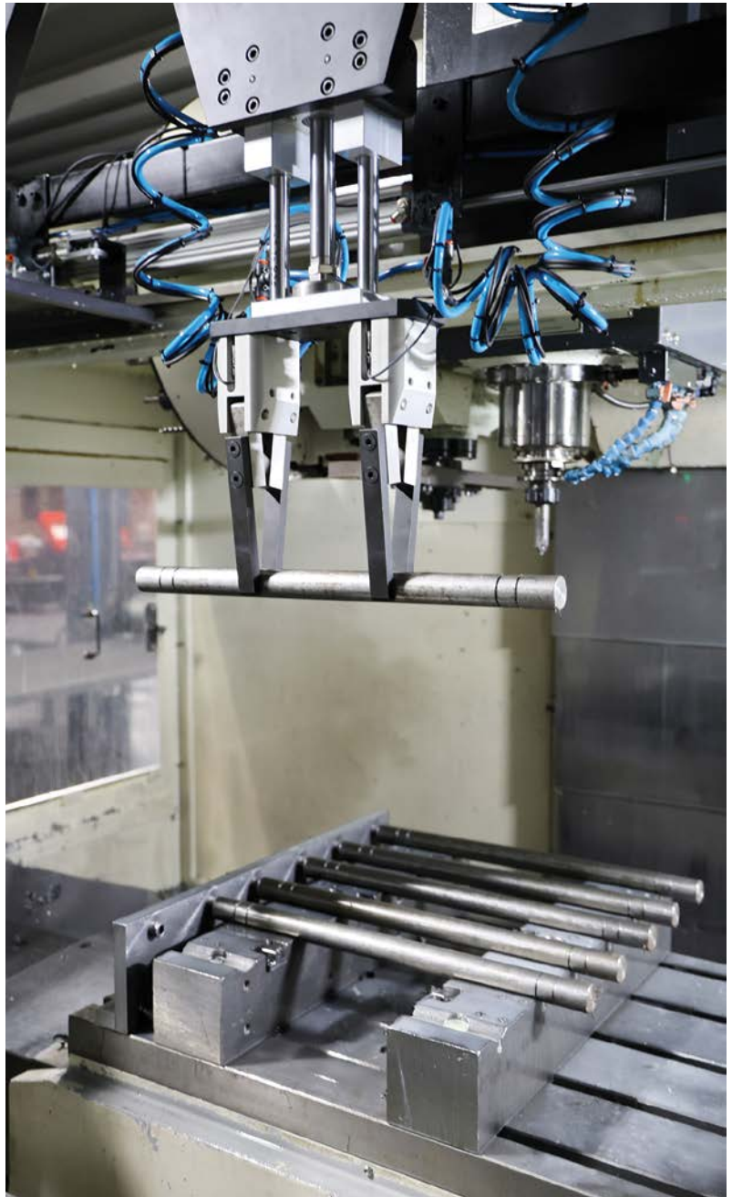
Automation of shaft machining for polyurethane rollers.
