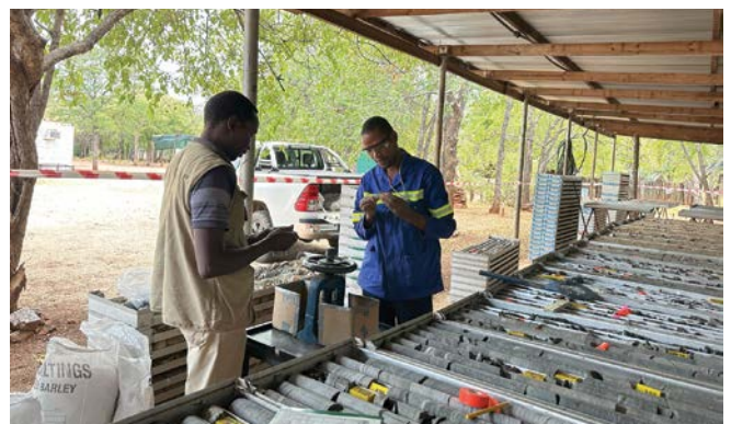
Sampling drill core at the warehouse facility.
