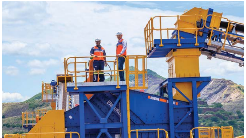
Above: Enduron screens installed as part of the beneficiation process at a local iron ore mine.
