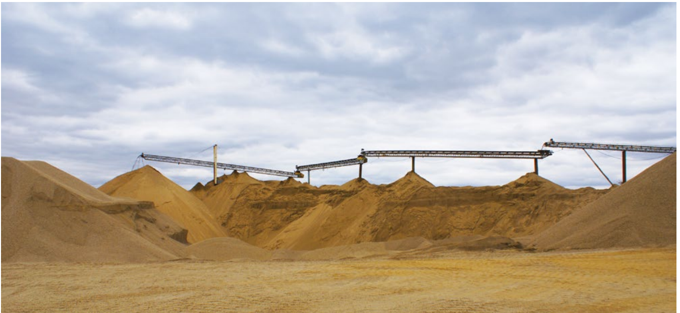
Inland sand is extracted and placed in stockpiles for transport to the processing plant.
