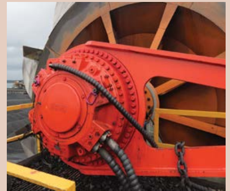
Hägglunds Drives provides drive solution for RBCT stacker reclaimer.
