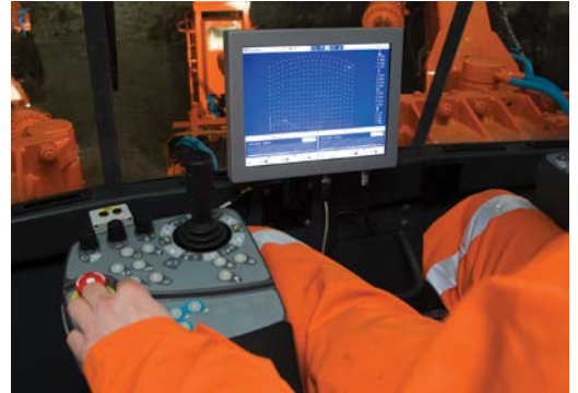
iSURE® allows users to run automated drilling cycles.
