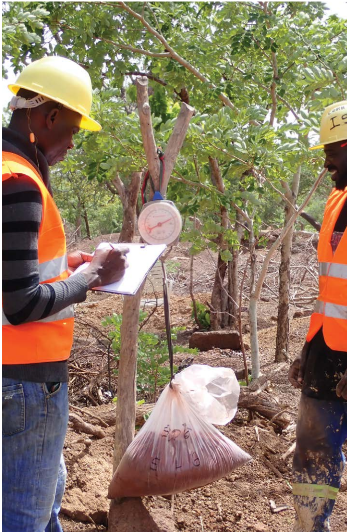
Soil sampling and weighing underway.
