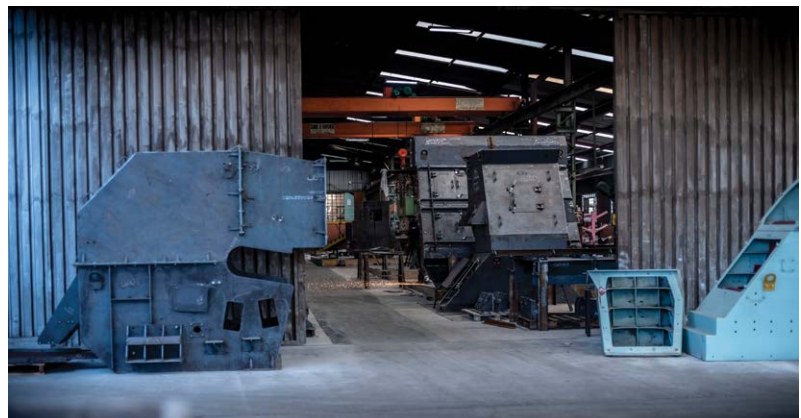
Chutes being manufactured in the Weba Chute Systems facility in Germiston, where each design is customised to specific applications.
