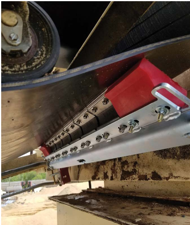
Tru-Trac belt scrapers keep conveyors running smoothly and are essential for reducing misalignment caused by material carryback.
