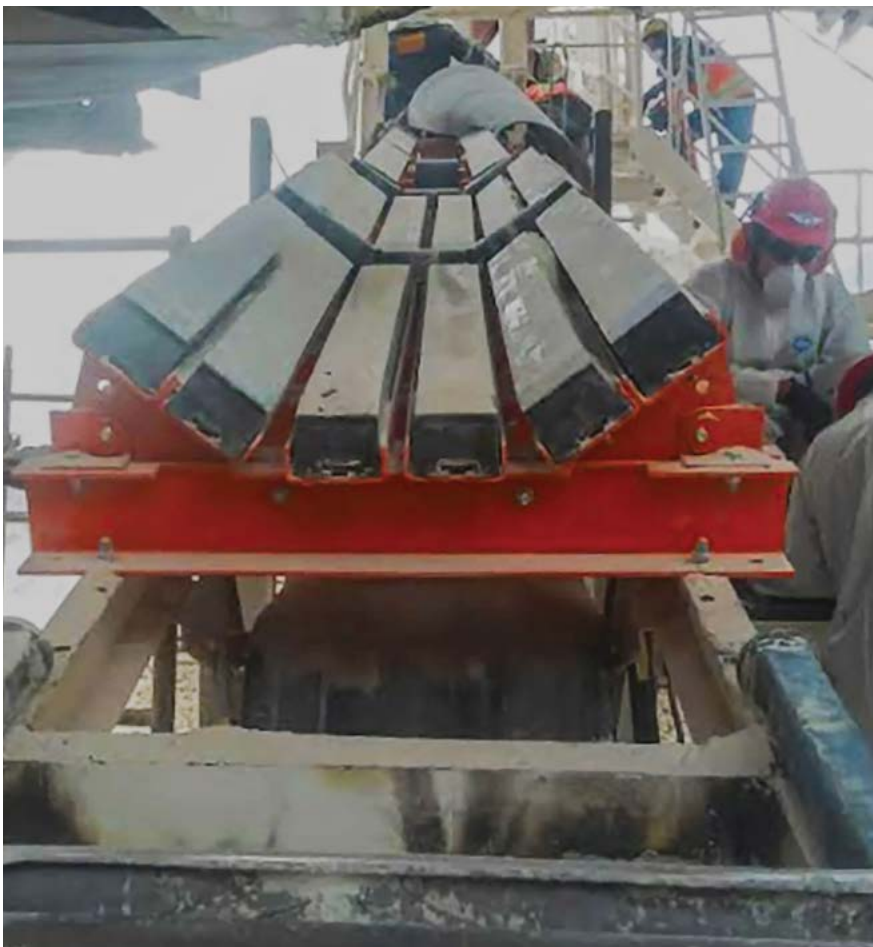
Cradles offer low friction surfaces at specified trough angles for superior belt sealing.
