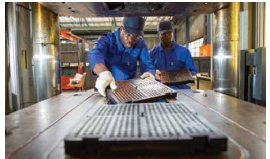
Multotec's flame-resistant rubber screen panels are available in hard (PD70) and soft (PD45) durometer rubber.
