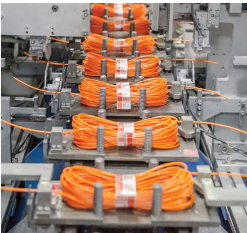
TS Initiation systems manufacturing detonators.
