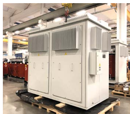
Trafo Power Solutions is one of the few local transformer specialists who can design and supply dry-type transformers in enclosures that meet IP65 rating.
