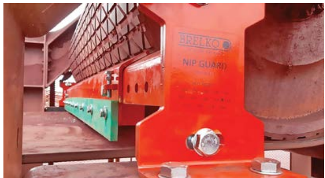
Brelko Nip Guard installed at Khumani mine.
