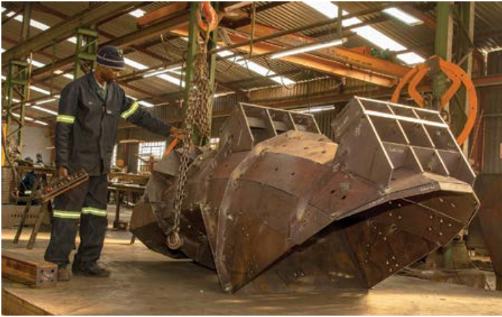
Weba transfer chutes being fabricated at Weba Chute Systems' facility in Germiston.
