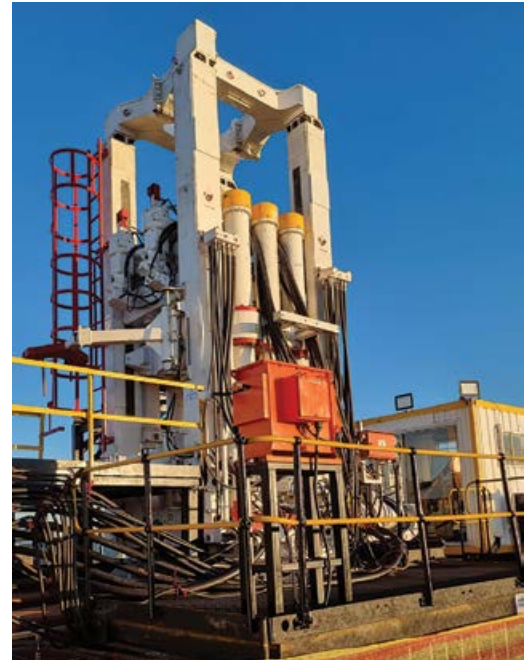
At the completion of the hole, a depth of over 950 m, the results showed that the drilling team was not more than 0,05% off its closure distance.
