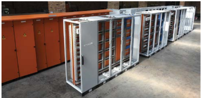
Electrical and control panels as work-in-progress on the factory floor.
