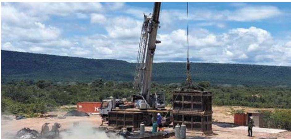
Stacked coking ovens 'cooking' the coal at 900-1100°C.
