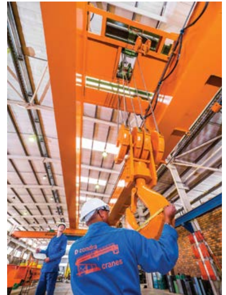
Typical overhead crane under test in Condra's factory.
