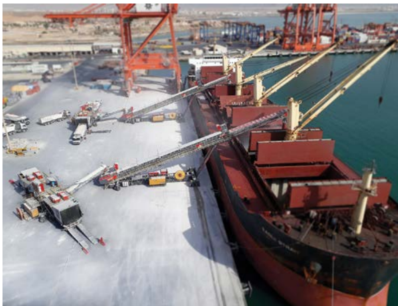
Telestack's efficient shiploading system.
