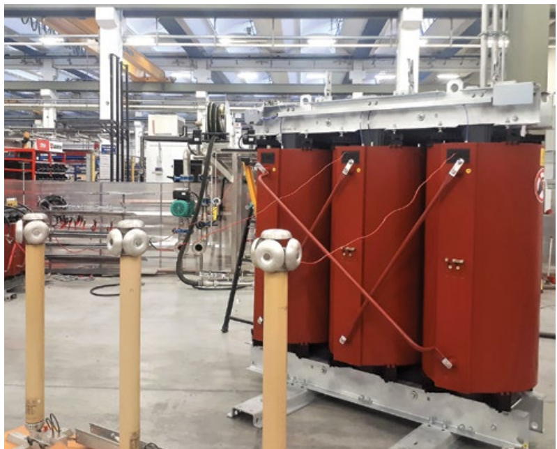
Partial discharge testing being carried out on a 1000 kVA dry-type transformer for a mining project.
