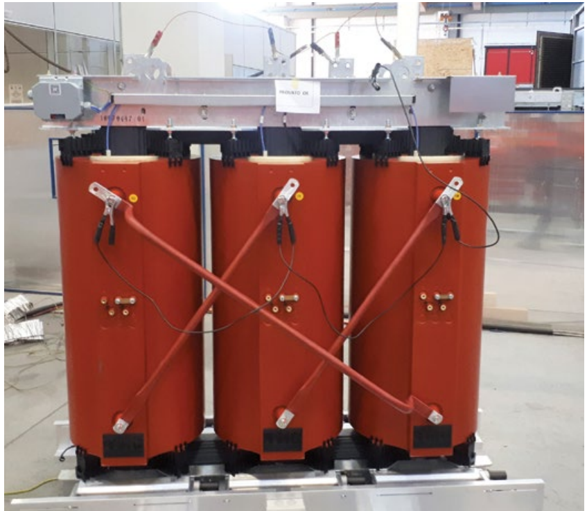
A 1000 kVA dry-type transformer going through the applied voltage test.
