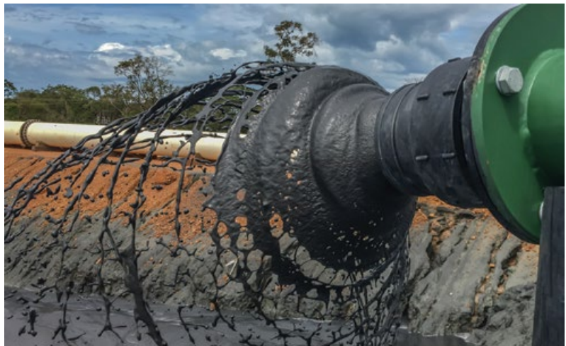
Multotec provided an innovative hydrocyclone solution for a safe and cost effective tailings storage facility at a large copper mine in Zambia.
