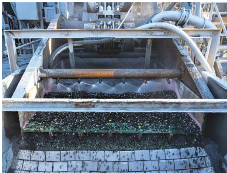
Primary Mill Discharge Screen.
