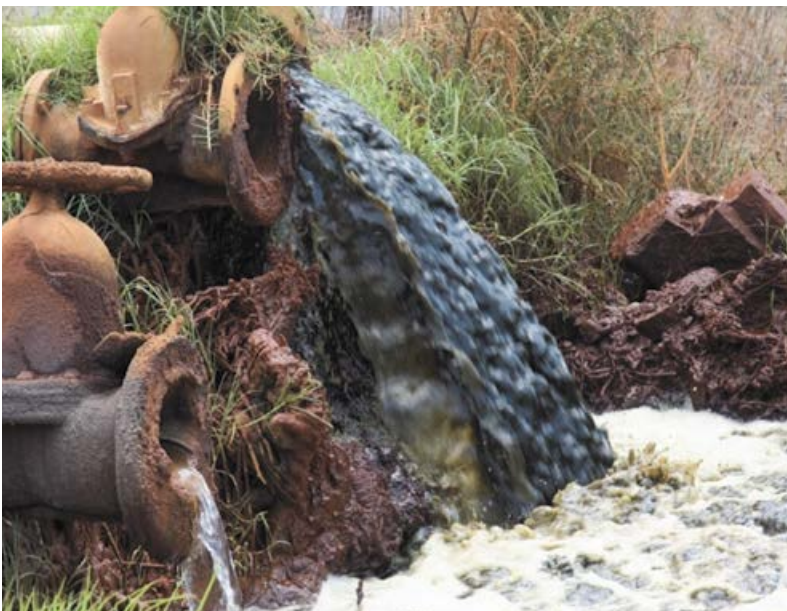
AMD contains a high level of dissolved salts, is acidic and comprises a wide spectrum of heavy metals in toxic concentrations.
