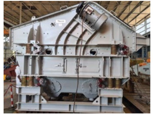
One of Kwatani's smaller screens used in diamond mining fitted with torsional springs.
