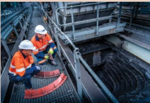
Components are installed once the wear rate is near 100% with a 10% confidence level still in place.
