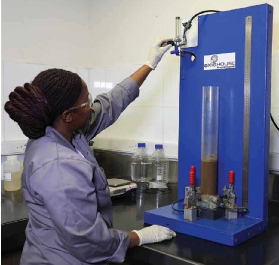
The froth column test is used to compare frothers in terms of froth rise rate, stability and rate decay.
