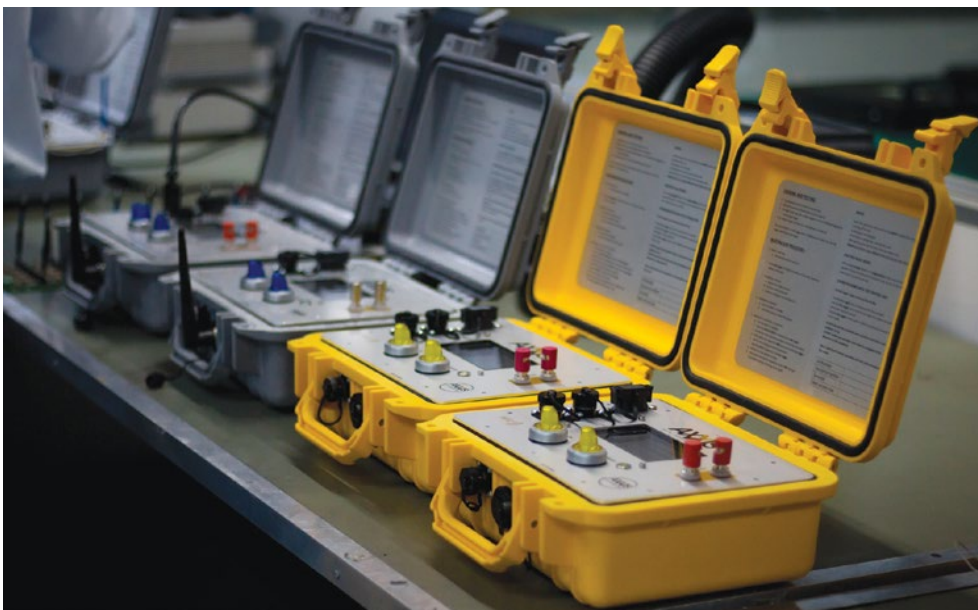
AXXIS Titanium allows mines to program blasts of up to 35 seconds long for larger and more complex.
