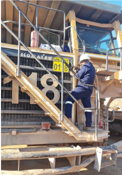
A Booyco Engineering HVAC system being installed on a mining vehicle.
