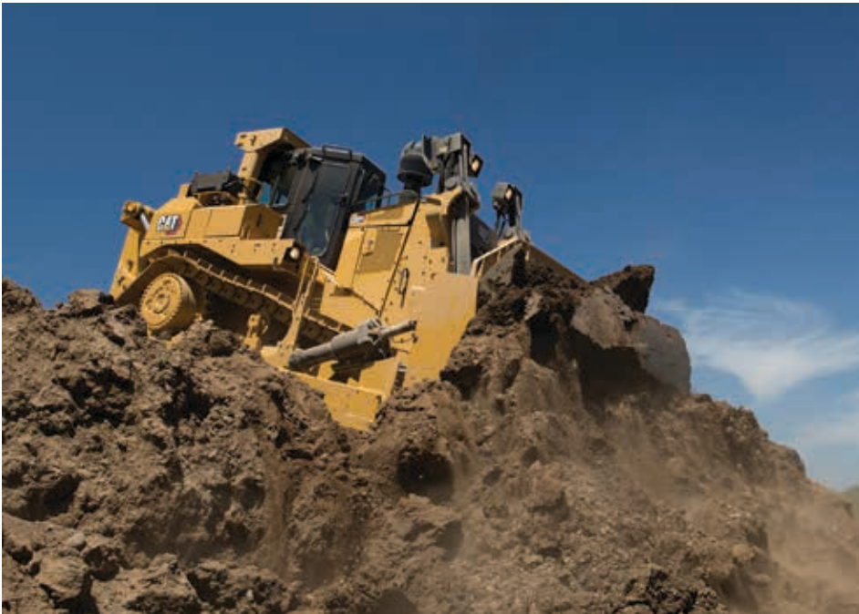
Cat D9 GC dozer dozing down steep slope.
