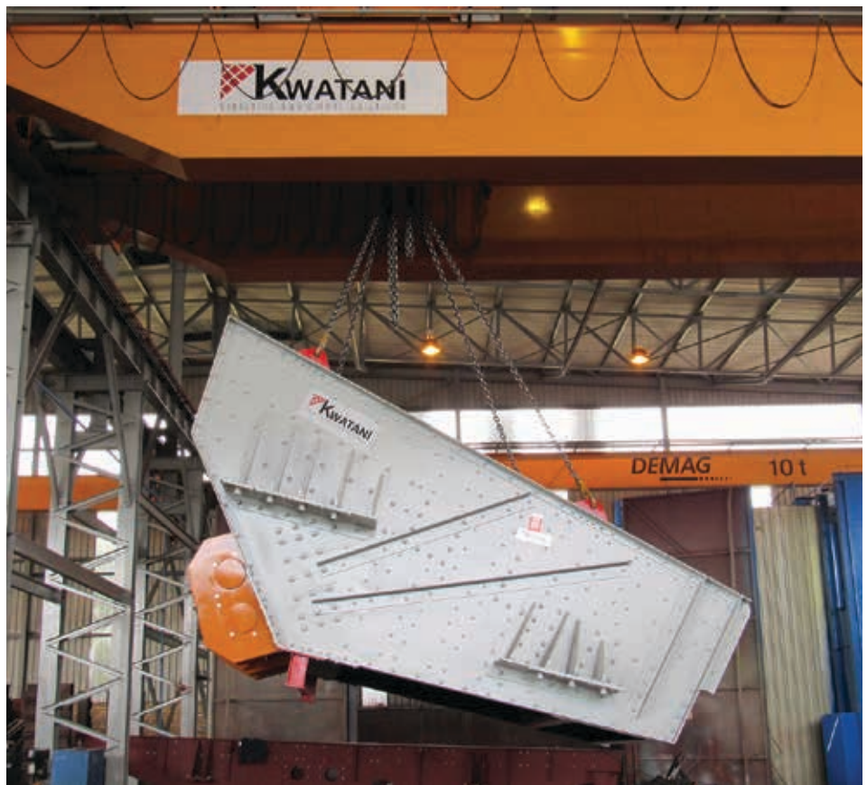
Kwatani designs and manufactures robust grizzly coal screens.
