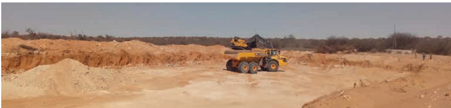
The mining fleet will consist of three production teams, each comprising one 75-t excavator and three 40-t articulated dump trucks.
