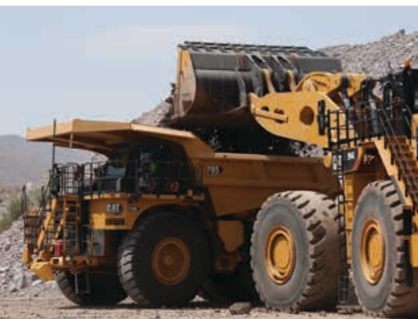
The Cat Next Gen 785 mining truck being loaded by Cat 994 wheel loader.
