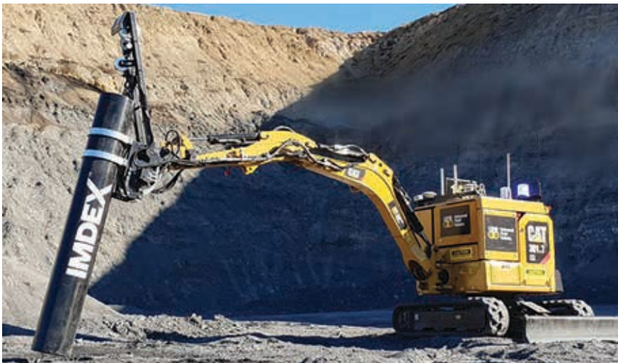
IMDEX Blast DOG is a semi-autonomously deployed system for logging material properties and blast hole characteristics at high spatial density across the bench and mine and is commodity agnostic.
