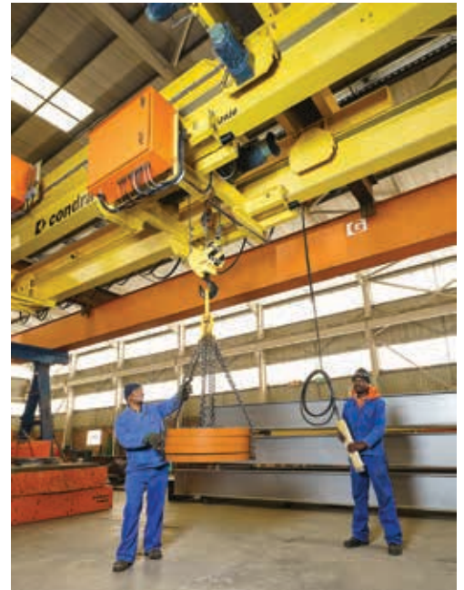
Condra crane with extendable boom, similar to the one recently ordered from North Coast Cranes & Lifting for a furnace application, seen here under test in Condra's Johannesburg factory.
