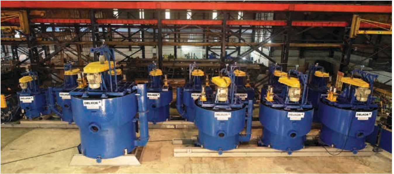
DELKOR BQR flotation cell with MAXGen mechanism.
