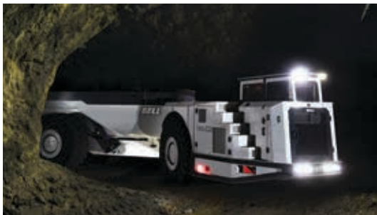
To achieve a more practical layout, product designers listened to customer feedback and moved from a centre-mounted cab to a left-hand side mount.
