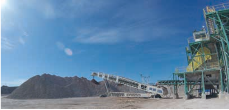
The heavy-duty RS radial stacker range from ABHS offers belt widths up to 1800 mm wide and works at production rates up to 5 000 tph.
