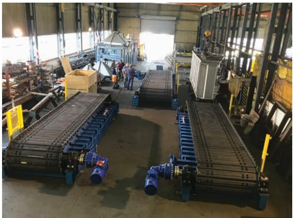
Apron feeder testing before shipment to Guinea.
