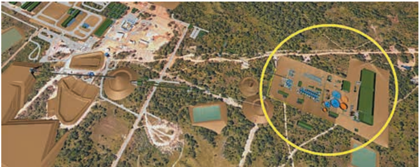
Screenshot of the 3D engineering model of Kakula's surface infrastructure, including the ore conveyor, run-of-mine ore stockpiles and processing plant (circled in yellow).
