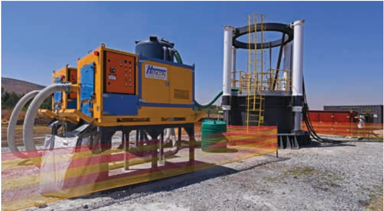
The 'front end' of the SBS with, on the left, the vacuum units.
