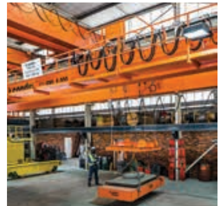
Overhead crane and hook-block undergoing load test prior to shipping.
