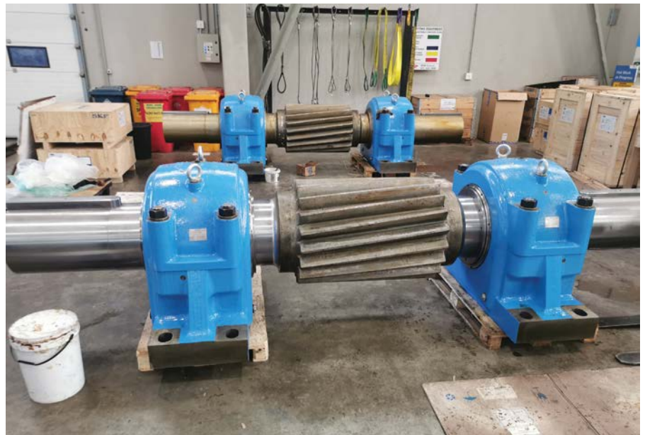
For horizontal grinding mills, SKF South Africa can custom-engineer and locally manufacture mill pinion housing assemblies.
