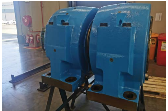
Left: Locally manufactured trunnion housing assemblies. One housing has been remanufactured, and the lead time has been reduced from 10 weeks for new production to 3 weeks for remanufacturing. Right: A set of SKF plummer block housings for mill pinions that were custom-designed and manufactured in South Africa.
