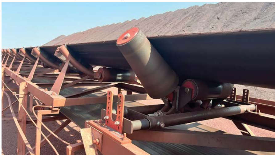
Tru-Trac trackers correct belt misalignment, preventing costly spillage and edge damage while keeping conveyor systems running smoothly.
