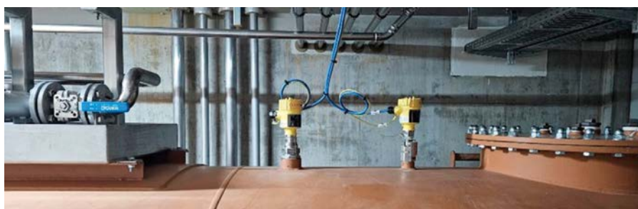
The tightly focused measuring beam of the VEGAPULS 6X radar level transmitter with 80-GHz technology allows installation with small process fittings.
