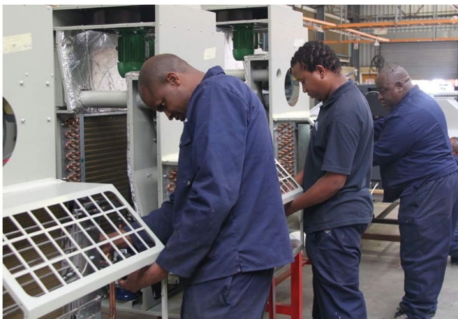
Booyco assemblers finalising construction of bespoke Booyco HVAC systems destined for the railway sector.
