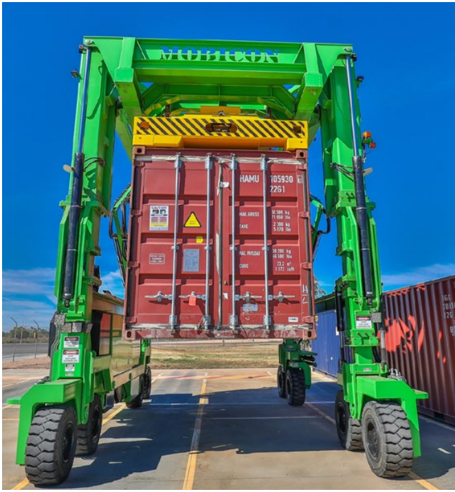
Mobicon mobile straddle carriers are designed for versatile container and product handling in and around automotive assembly plants.
