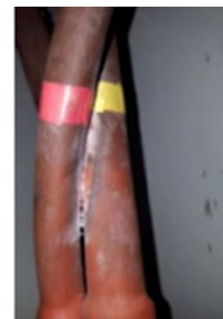
Left: A PD graph on medium voltage (MV) terminations trended over time. The escalation in Q_{max} (mV) as the resistance of the insulation deteriorates is evident until failure occurs, which trips the supply voltage. Right: Typical partial discharge (PD) failures owing to inadequate clearance between the unscreened areas of the cable termination. PD causes the build-up of a white acid-type powder due to the ionisation of the air around the activity.
