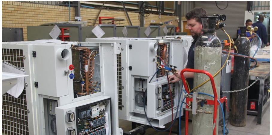
Final quality inspection of Booyco HVAC systems, which are built to withstand excessive vibration, shock loading, dust and extreme temperatures.
