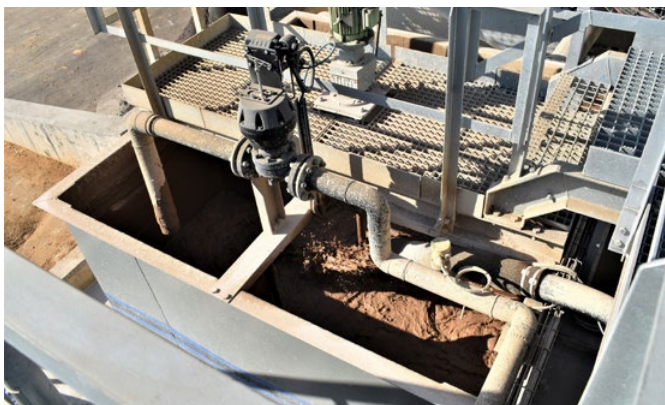
Left: The top of the lime buffer tank where lime is stored during the slaking process. Right: With water recovery of between 98% and 99.5%, the only liquid to leave the plant is the moisture in the dewatered sludge.
