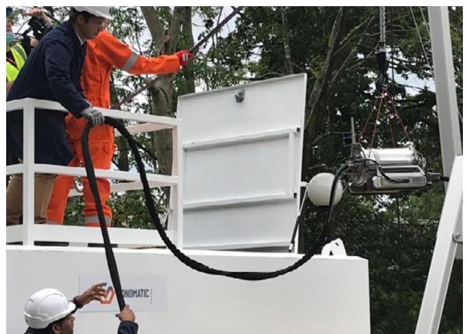
The nautilus robot's design offers the smallest possible footprint to allow entry to liquid storage tanks via small manholes.
