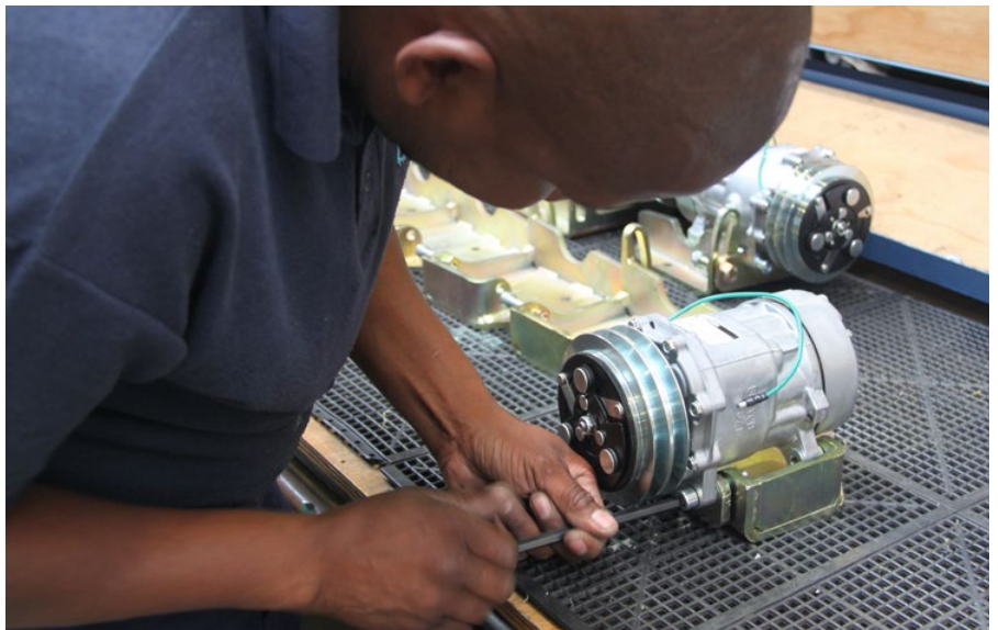
Completing a Booyco refrigerant compressor assembly used on many military and mining systems.
