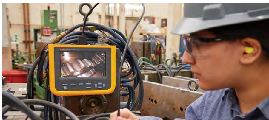
High-resolution videoscopes allow industrial maintenance teams to quickly identify equipment issues and schedule preventive maintenance.
