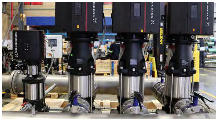
Left: Grundfos XL CR systems combine hydraulic efficiency with high efficiency IE3 motors making them ideal for use in water treatment plants and pressure boosting stations. Right: For high flow applications, Grundfos can also supply large multiple pump solutions of up to six pumps, and each pump will only run at the speed required to meet demand.
