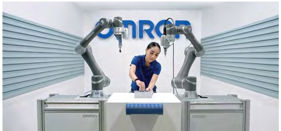
The Omron Techman TM14M robot can lift goods up to 14 kg. It brings innovation to the factory floor through true harmonisation and collaboration between humans and machines.
