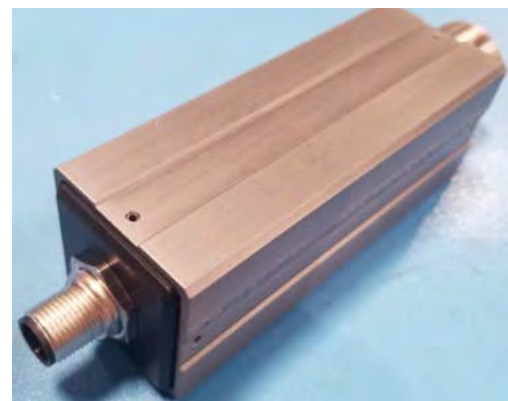
H 2 scan's Gen5 System for dissolved gas analysis (DGA) of hydrogen in transformer oil, which is now available in South Africa from RTS Africa.
