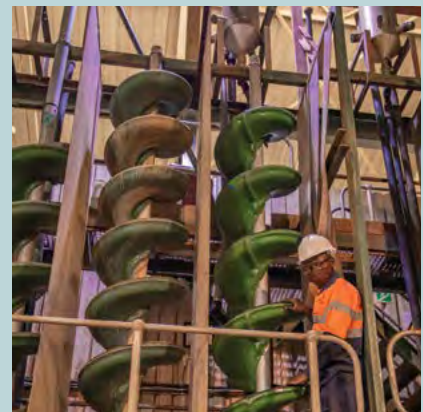
Hlayisi Baloyi, applications engineer at Multotec, has been conducting extensive test work on Multotec’s new SC25 spiral concentrator using ferrochrome samples from numerous mines.
