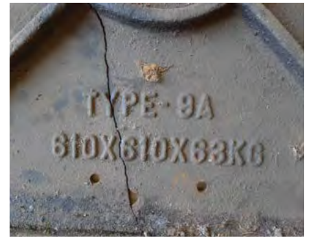
Left: Brittle fracture in crystalline materials like steel operates by cleavage, where the grains cleave or split along preferred planes within the crystal. Right: Brittle fracture is characterised by its sudden onset and an almost complete lack of plastic deformation. This man-hole cover, designed for foot-path use, was accidentally installed on an airfield apron, and failed when a jet taxied over it.
