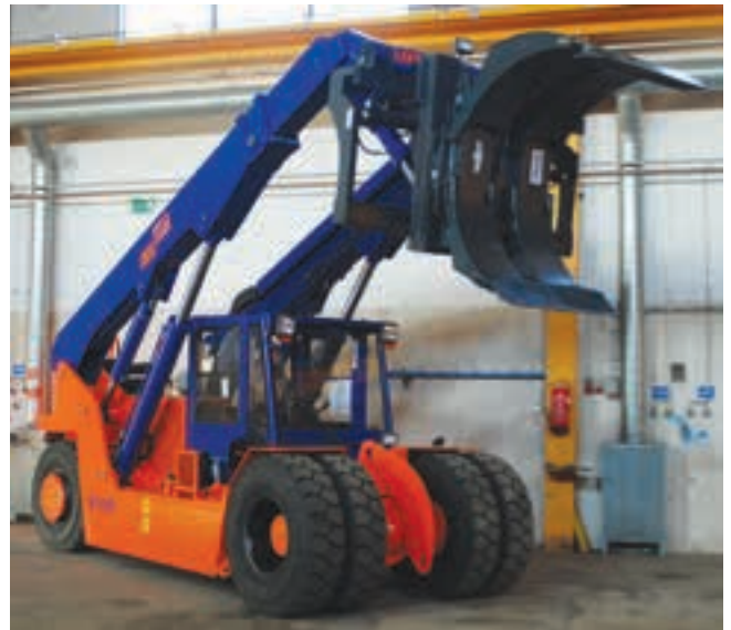
Meclift variable reach truck with paper clamp attachment for efficient handling of paper rolls.
