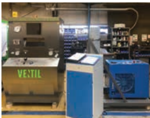
The pressure relief valve test bench use by Brimis.
