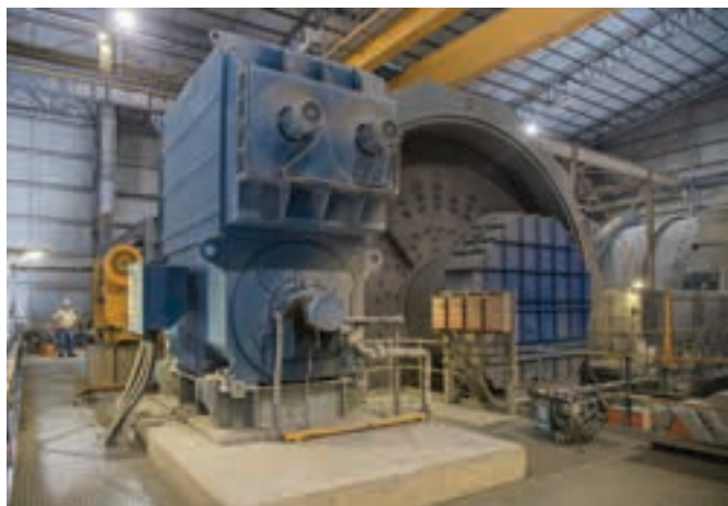
A high voltage mill drive motor in operation at a mine in South Africa.
