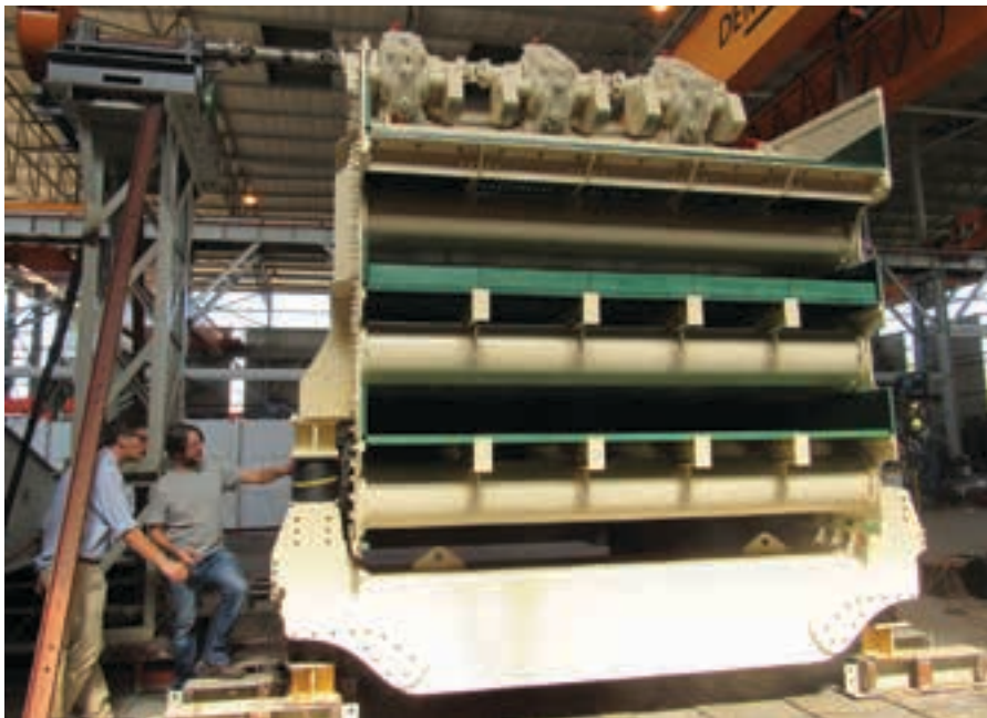
A large Kwatani triple deck screen for a diamond mine.
