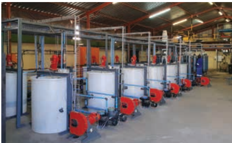
Trailblazer Technologies' recovery-based water treatment process uses a battery of continuously stirred tank reactors (CSTRs) and operates continuously and counter-current to produce demineralised water, with the contaminants being absorbed onto the ion-exchange resins for recovery upstream.
