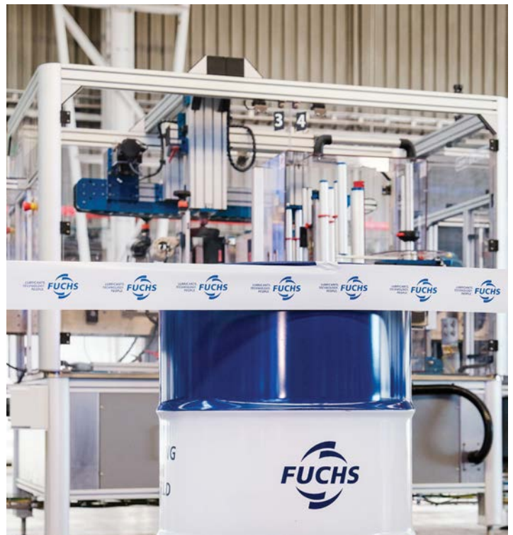
The three new filling lines increase throughput for bulk filling, IBCs, and drums, as well as 20 L pails, and smaller packs.
