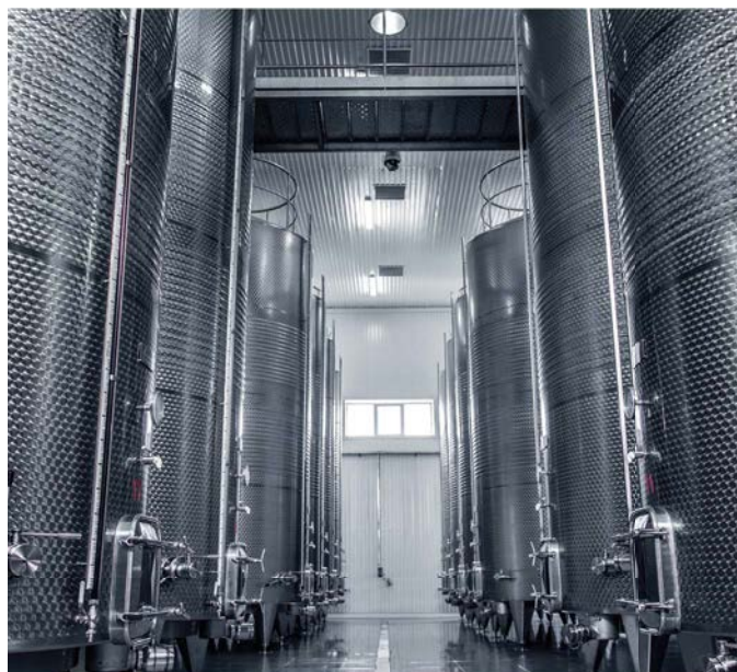
Used in tanks that can be up to 10 metres high, for example, the LW2720 sensor provides precise level detection.
