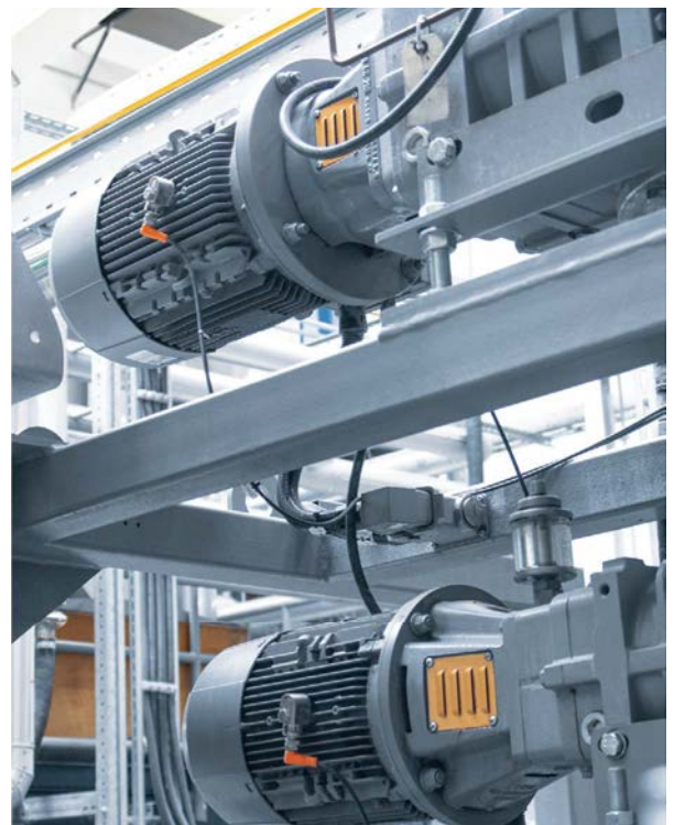
Up to 80 vibration sensors are installed in a current EREMA system. They monitor, for example, the motors and gears of the system.
