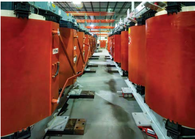
Precision-engineered cast resin transformers in the TMC production plant – ready for testing and final quality inspection.
