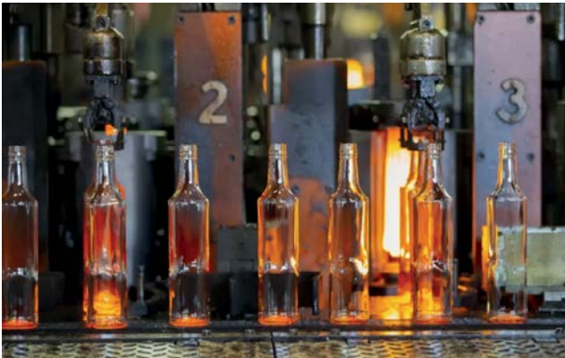
Left: The reflective nature of molten glass complicates temperature readings as varying emissivity can lead to measurement inaccuracies. Right: Real-time monitoring provided by IR technology enables immediate adjustments to be made during the production process.
