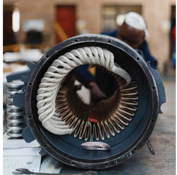
Hexagon Electrical manufactures customised, high-performance specialised electric motors. Pictured here: winding of a flameproof water-cooled motor.
