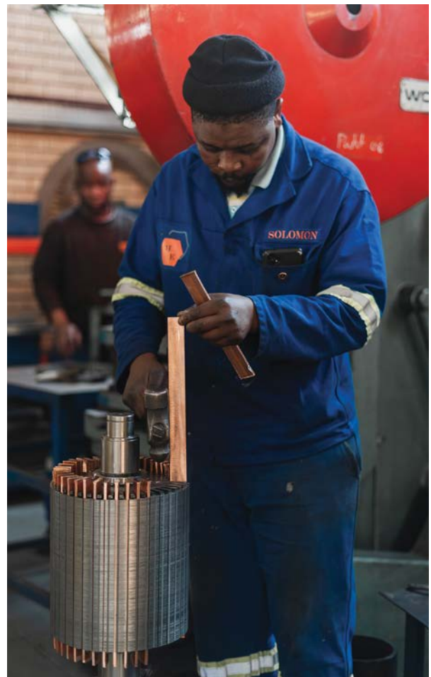
Barring a new copper bar rotor in the production workshop.
