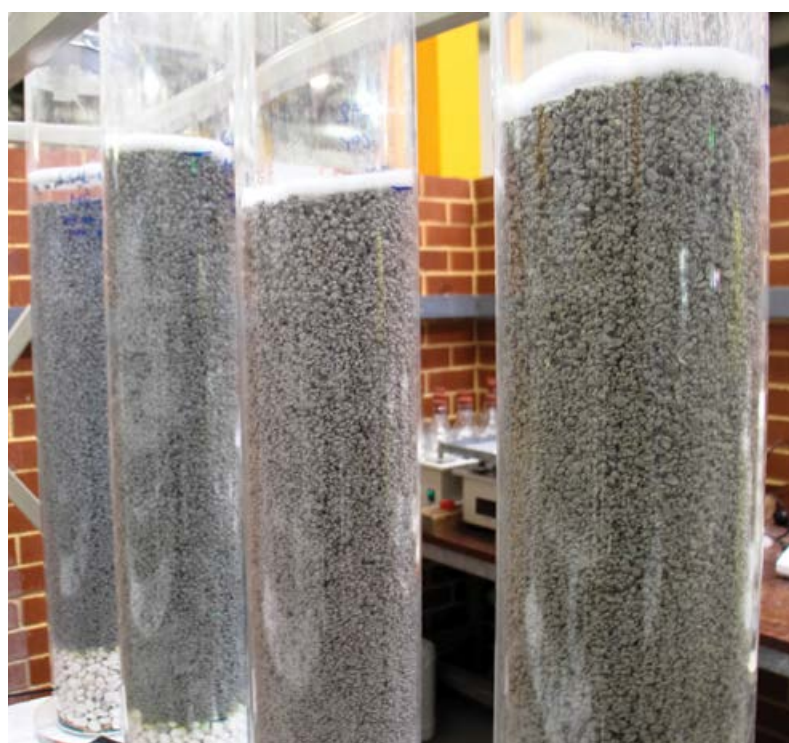
Mini-columns used to do initial discovery tests for heap leach amenability.
