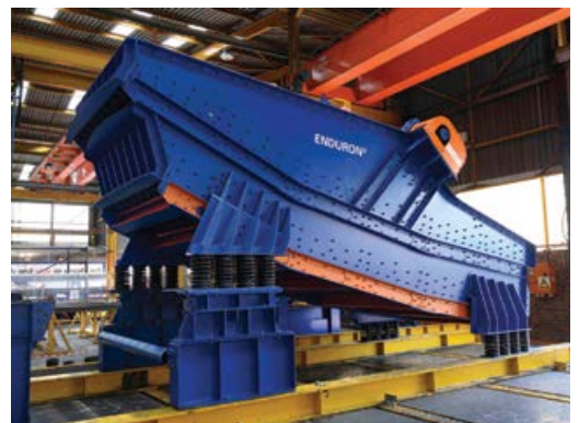
Weir Minerals in South Africa is the technology hub for designing Enduron vibrating screens which are locally manufactured.
