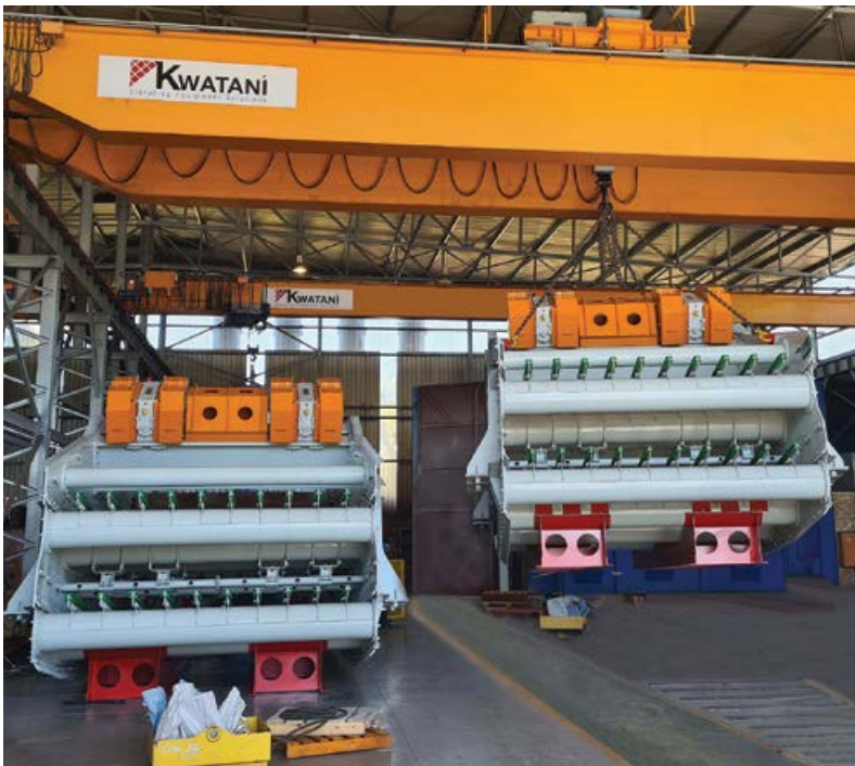
Kwatani double deck banana screens for a crushing plant.
