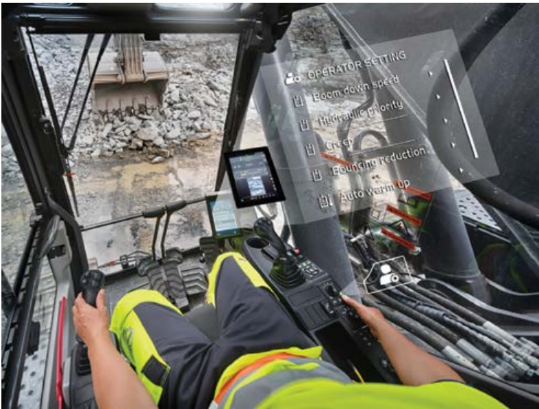
Operators can easily select and adjust a number of functions depending on personal preferences and the task at hand.
