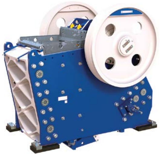
Another development has been the introduction of the larger Jaw Crusher Pro models with improved nip angles and stroke.
