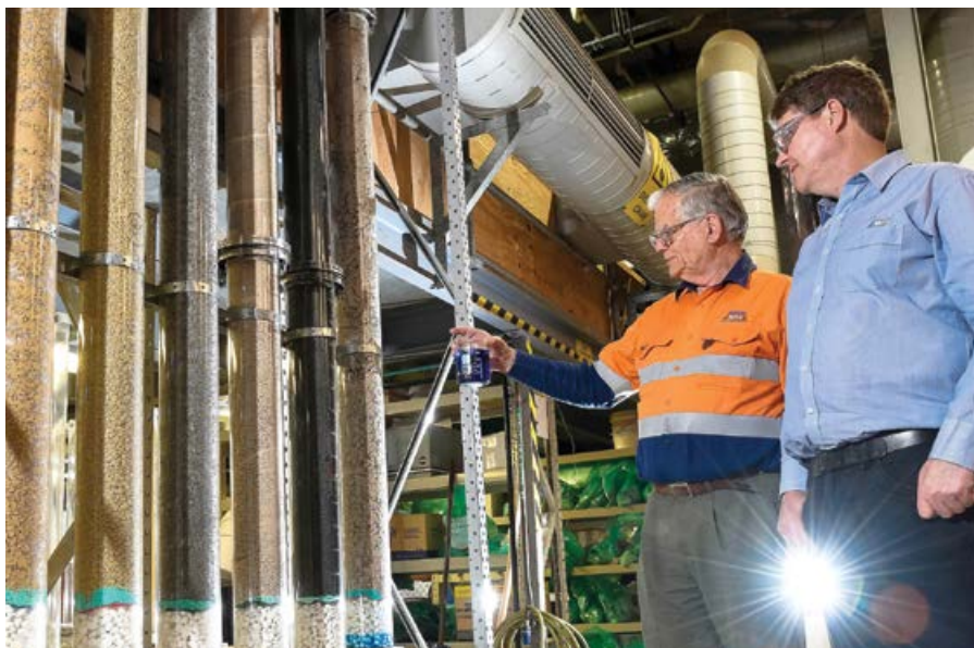
6 m columns fully loaded and used to confirm heap leach parameters.
