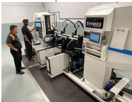
Coilshop Manager, Shawn Teixeira (left) and Operator, Mbukeleni Musibuko, with the new automated CNC coil spreader machine.
