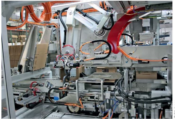
The highly automated packaging machine features a case feed robot inside to move flat corrugated cardboard into the case erecting segment.
