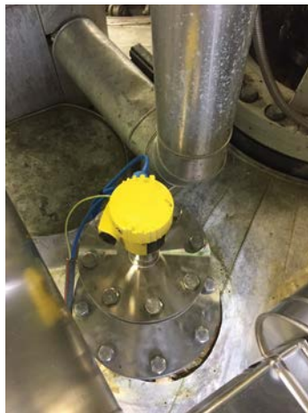
Electronic differential pressure measurement with VEGABAR is silicone oil-free, without capillary lines and requires less installation effort.
